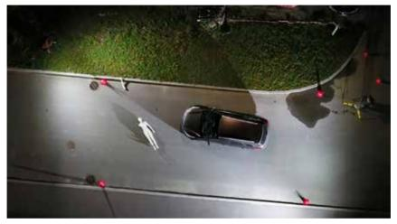
FIGURE 5: A 45 mm focal length RGB camera orthomosaic and point cloud, geo-referenced using RTK GNSS.
