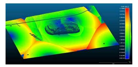
FIGURE 11: An accuracy assessment of a 45 mm focal length RGB camera point cloud (data product-4, geo-referenced using the drone's onboard GNSS), against terrestrial scanner benchmark data in the two-dimensional direction (x and y).
