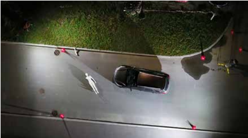
FIGURE 5: A 45 mm focal length RGB camera orthomosaic and point cloud, geo-referenced using RTK GNSS.
