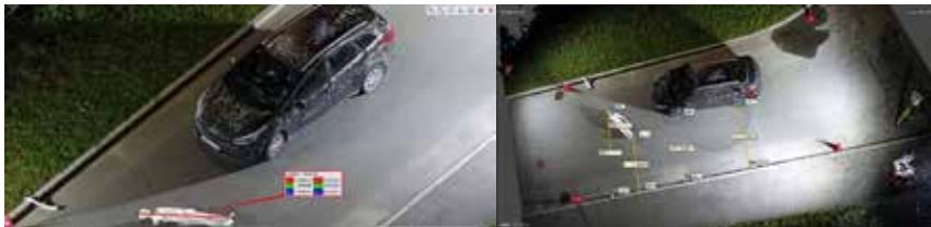
FIGURE 12: A 45 mm focal length RGB camera point cloud (geo-referenced using a scale bar), showing the measurement of the control scale bar (on the left) and the check scale bar (on the right).
