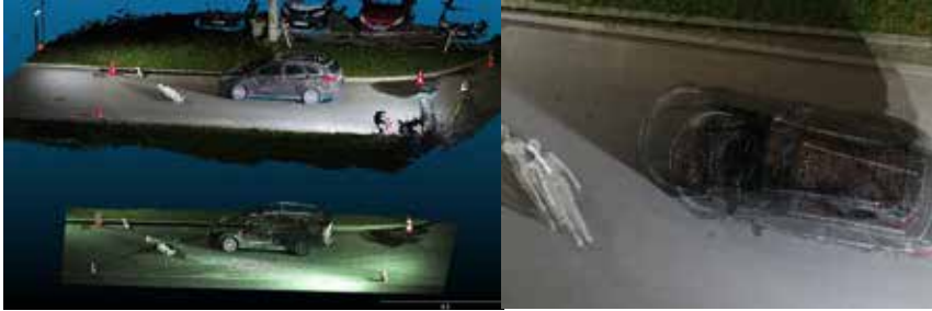
FIGURE 9: An accuracy assessment of a 45 mm focal length RGB camera point cloud (data product-4, geo-referenced using the drone's onboard GNSS), against terrestrial scanner benchmark data.
