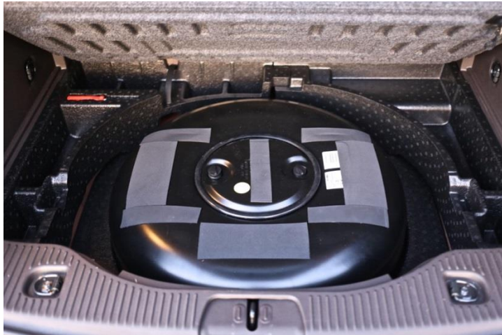
Joonis 8. Gaasiballooni paigutus varuratta asemel (Haymarket Media Group, 2018)
